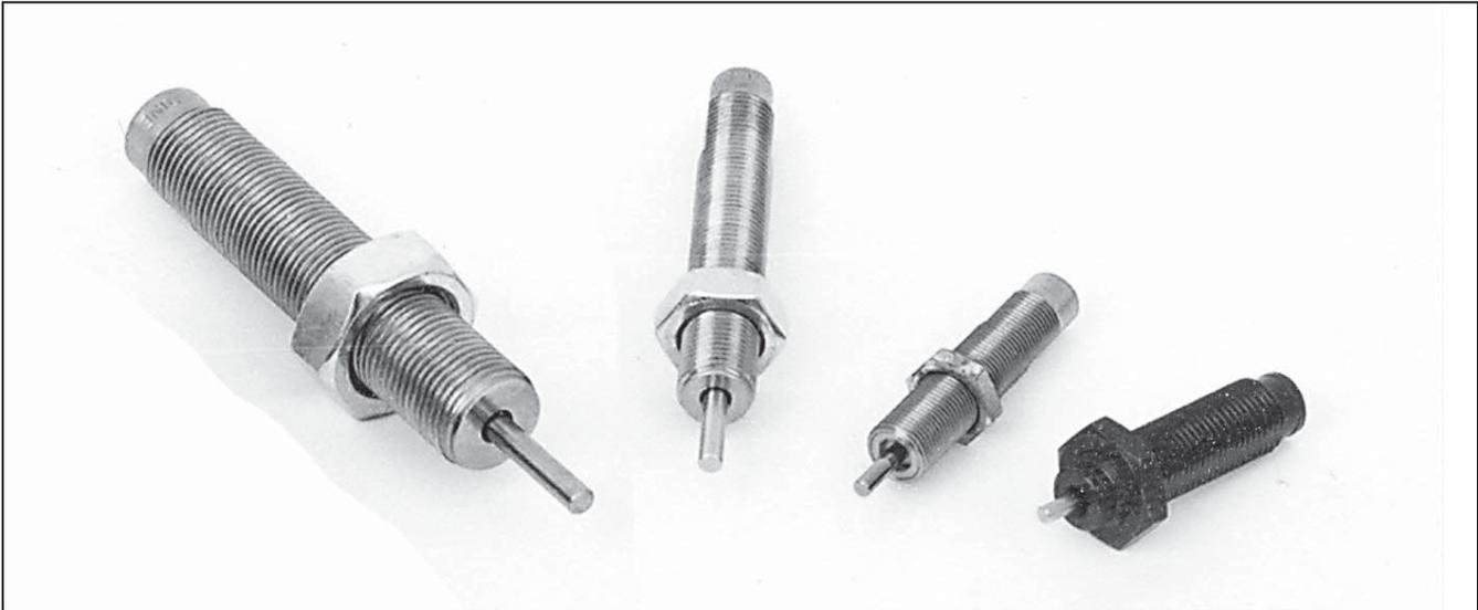
The progressive damping characteristics and built in "self compensation" design, decelerates a moving mass by minimizing the reaction force at impact and gradually increasing the resistance force throughout the working stroke of the shock absorber. (i.e.: higher speeds with softer stops)
