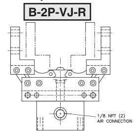
Note: **R** indicates that the position of ports and mounting holes are rotated 90° from standard version as shown above.
