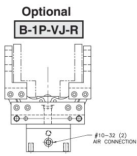
Note: **R** indicates that the position of ports and mounting holes are rotated 90° from standard version as shown above.
